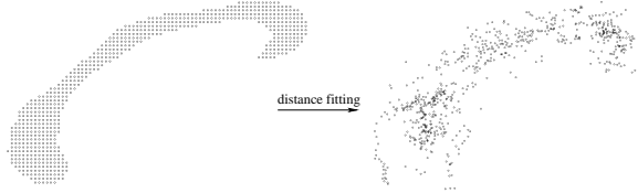
Figure 4: Seed points are adjusted so that Euclidean distances between the points on the plane reflect the distances between their associated integral curves.
