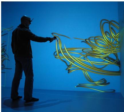
Figure 2: A user interactively seeds particle traces in an immersive virtual environment.
