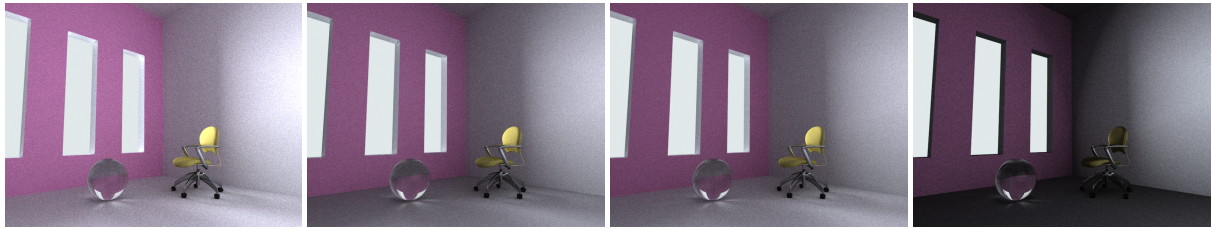
Figure 3: Pathtraced room scene using different diffuse models. From left to right: Lambertian, Wolff, Oren-Nayar, Ginneken et al.
