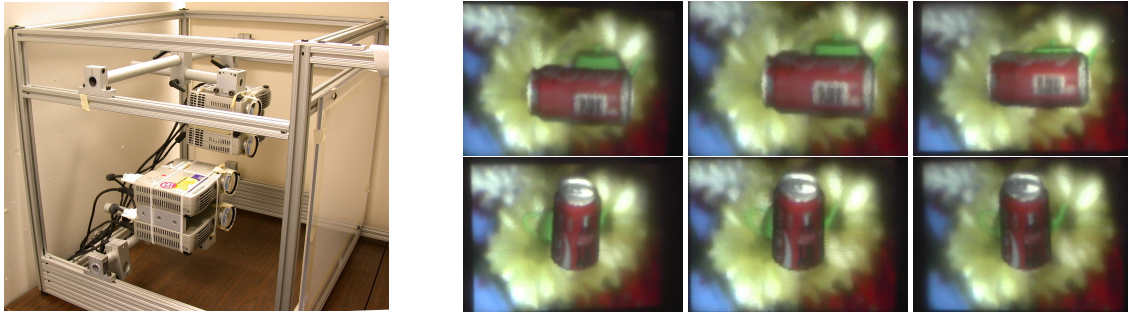
Figure 1: (Left) A prototype light field display composed of four projectors. (Right) View-dependent effects from the prototype. These images are captured with a regular camera from different viewpoints. The scene contains a Coke can, a teapot, and a textured background. The Coke can is rotated in the second row of images.
