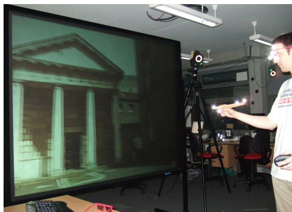
Figure 1: System setup. Two of the Vicon cameras can be seen in the background. The bright glares are the reflective markers.
