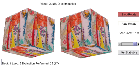
Fig. 1: Each cube face is 160^2 pixels. (Left) Texture of 144^2 pixels interpolated to 160^2 pixels. (Right) Original texture resolution of 160^2 pixels.
