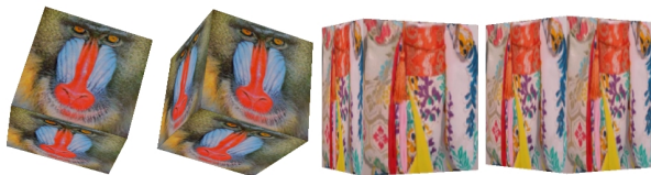
Fig. 9: Test level 160: LHS is 160 and RHS is 75% resolution interpolated. It can be seen that the baboon and kimono texture quality on both cubes are similar.
