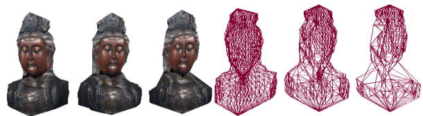
Fig. 10: From left to right, the queen models, textured mapped and mesh, have 1296, 900 and 542 vertices respectively.
