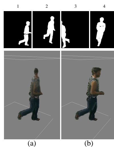
Figure 1: Differences in 3d shape reconstruction when objects do not project themselves onto all images: (a) using already published SFS methods; (b) using our modified SFS algorithm. Voxel coloring, done using backward raytracing, is only given for image comprehension.
