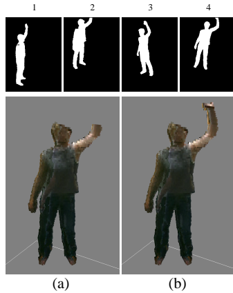
Figure 6: Voxel based shape estimation for a complex object: (a) shape computed by original SFS algorithm; (b) using our extended SFS algorithm.
