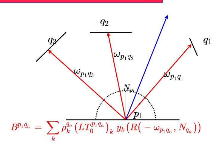
We compute interreflection by finding hitpoints about a given surface position  $(p_1)$  obtained from the UV-mapped Surface points  $(G_p)$ . For each hit-points  $(q_i)$  we calculate radiance contribution at  $(p_1)$  [we fetch  $(T_{qi})$  from previously calculated Transfer-texture $(T_0)$ ]. This is repeated for all such hit-points  $(q_i)$  to obtain an indirect radiance map.
