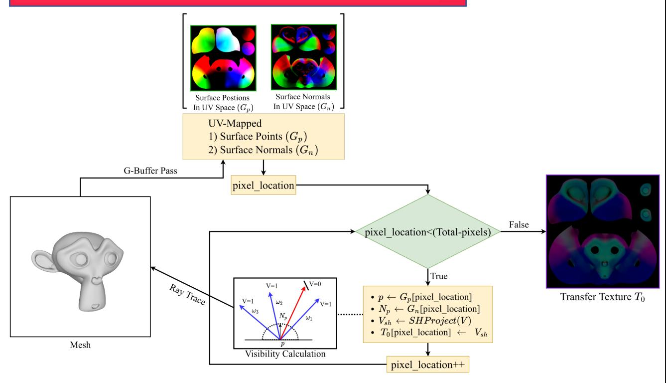
Given a mesh, we obtained UV-mapped surface positions and surface normal in texture space via G-buffer passes. For every pixel location, we obtain a surface position (p) and surface normal  $(N_p)$  we ray-trace to obtain visibility of (p) and project it to SH-basis. We do this to every pixel location to obtain the Transfer-Texture  $(T_0)$ .
