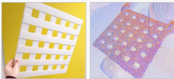
Figure 1: Shots of our 3D lattice target (left); our lattice represented by point clouds from multiple cameras after registration (right).
