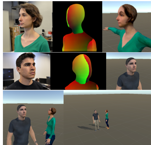
Figure 2: 3D reconstructed models. Here we apply the texture captured in the first step over the mesh generated by the second.
