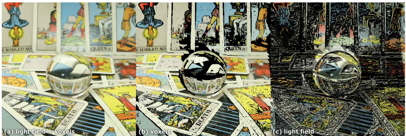
Figure 1: Hybrid rendering of light-field and voxelized light-field data (a). The original light field consumes 216.8 MB of memory (3 colors; 8 bit per channel), while our hybrid representation compresses the data to 82.4 MB (38%). Isotropic and uniform scene areas can be represented as voxels (color+depth), requiring only 0.5 MB of sparse data, without a perceivable loss of quality (b). Anisotropic scene parts (e.g. reflections and refractions) and occlusion boundaries (producing errors in depth reconstruction) are represented as sparse light field, requiring 81.9 MB of data (c).
