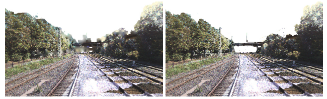
Figure 3: (a) [PGA11] visibility with push-pull filling. (b) our adaptive filling. (Linear parts have been removed on both)
