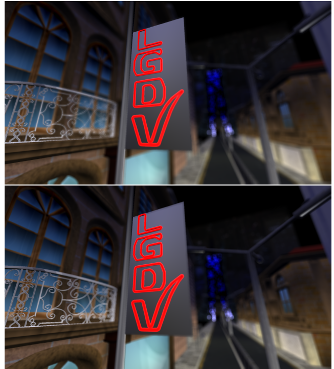
Figure 1: Standard filtered DOF (top) and our method (bottom). Note how with our method the railing is more clearly in front of the windows.
