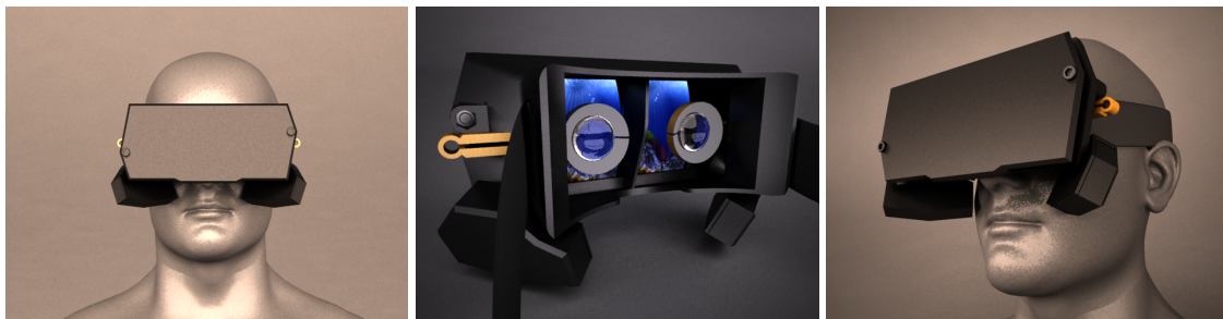
Figure 1: Visualizations of our HMD concept containing an integrated binocular eye tracking device.
