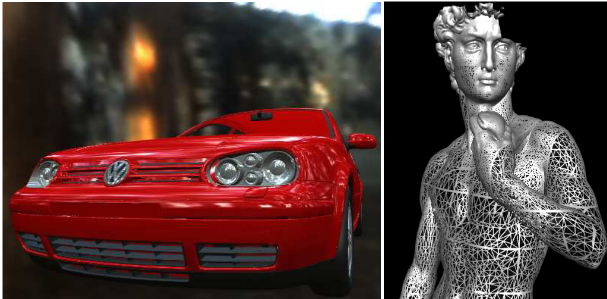
Figure 6: Results from the LOD rendering algorithms. Left: a car model consisting of about 8000 trimmed NURBS patches which are tessellated on-the-fly. Right: Out-of-Core rendering of the famous David model. Note that the missing part of the head was culled away since it lies outside of the view-frustum.
