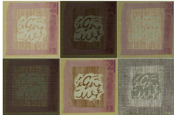
Figure 2: Six views of a wallpaper from various view and light directions acquired by our automatic material measurement setup. The appearance of the material changes drastically which is correctly represented in BTFs.
