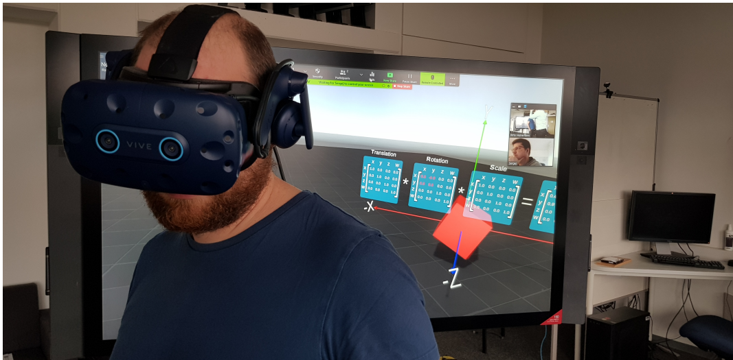
Figure 5: A test person watching the animated cube and the transformation matrix composition in the Application. From left to the right: Translation, Rotation and Scale multiplied into TRS matrix. Individual matrices were later coloured to allow better recognition.
