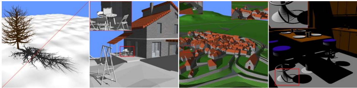
Figure 1: (from left to right) A tree rendered with a 1K \times 1K shadow map at 42 fps (upper left) and using alias-free shadow maps as proposed in this work at 3 fps (bottom right). The yard scene rendered with a 1K \times 1K shadow map at 60 fps and with alias-free shadows at 4 fps. The village scene rendered at 7 fps with alias free shadows. The kitchen scene rendered with alias-free shadows at 9 fps. In all three examples the resolution of the conservative shadow map was 1K \times 1K .
