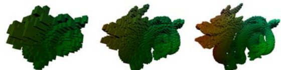
Figure 2: 3D rasterization of the Stanford Dragon at three different resolutions.
