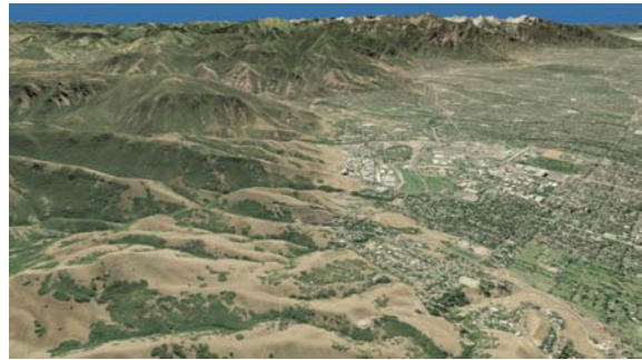
Figure 5: Screenshot of the Utah data set, rendered with the ray-caster. With an extent of 460 km \times 600 km at a resolution of 5 m and 1 m for the height field and texture, respectively, this data set amounts to 790 GB of data.
