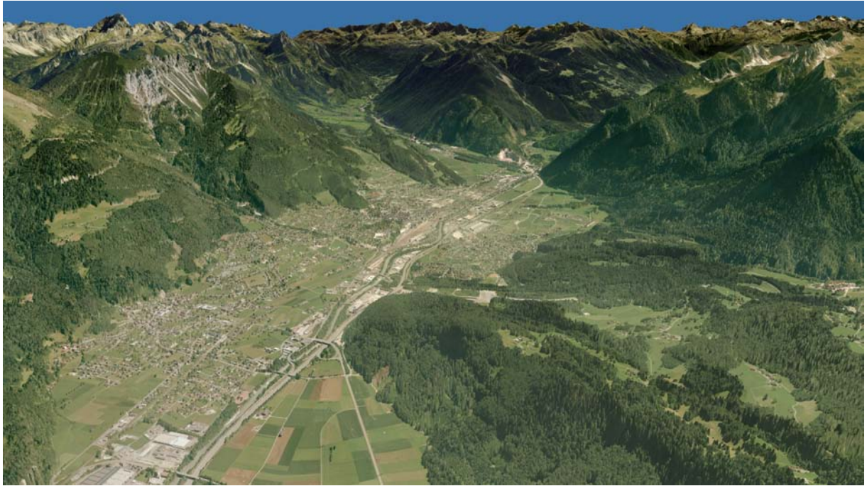
Figure 1: A textured DEM of Vorarlberg, Austria ( 56\text{ km} \times 85\text{ km} ) is rendered on a 1920 \times 1080 view port using our method. The spatial resolution of the DEM and the texture is 1\text{ m} and 12.5\text{ cm} , respectively. Even though we render to a 2 megapixel view port, an average frame rate of about 30 fps is achieved at a geometric screen-space error of below one pixel.
