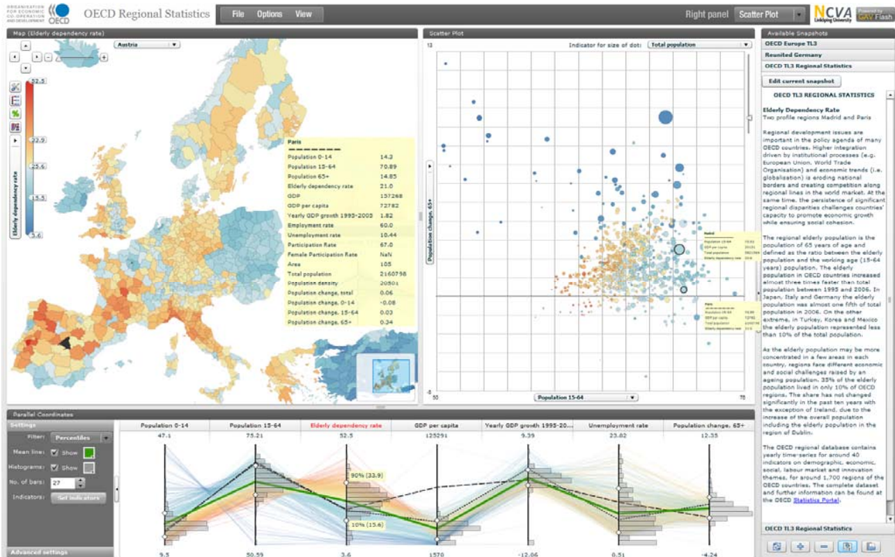
Figure 1: A snapshot of OECD eXplorer for Adobe Flash and Flex. The visual interface has three coordinated and linked views (choropleth map, scatter plot and parallel coordinate plot (PCP)). The coloured indicator is “Elderly dependency rate”, defined as the ratio of the population aged more than 65 years and the amount of people between ages 15-64. Two regions, Madrid and Paris, are highlighted in all views and their two profiles in PCP can be used for comparison including the distribution of the elderly dependency rate across the European regions. The extended PCP component includes statistical analysis functions (histogram and percentile-based filtering) attached to the indicator axes and can be used in the analytical reasoning process. The insight about the elderly dependency rate across OECD regions is here saved together with relevant metadata (see right view).
