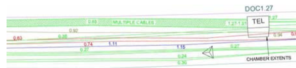
Figure 5: Cables extent to reduce clutter.
