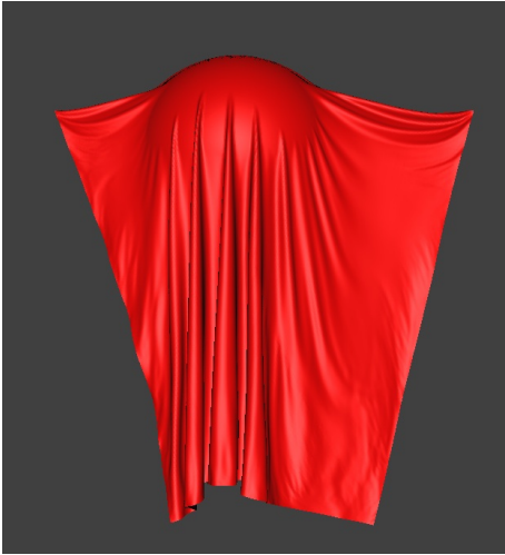
Figure 7: Simulation of a piece of cloth with 90K vertices at 20fps on a GPU using LRA.
