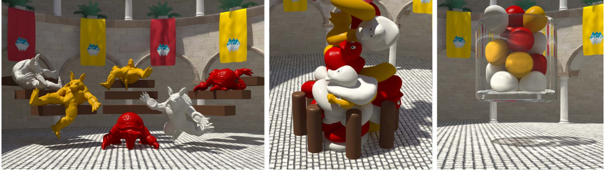
Figure 13: Robust and volume-conserving deformations using shape matching. Armadillos (32442 particles total), 20 ducks and 20 tori (21280 particles total) and 20 balls (7640 particles total) were simulated in real-time on a GPU.
