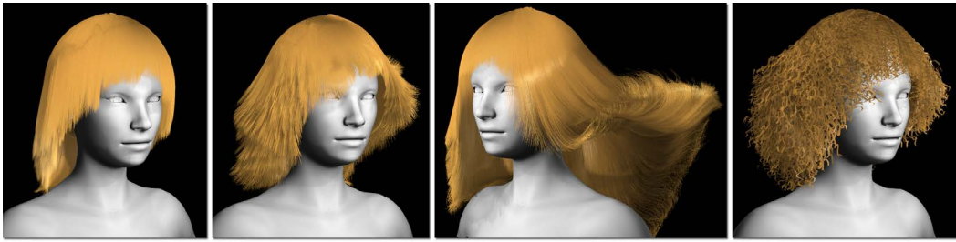
Figure 9: Dynamic FTL allows the simulation of every hair strand in real time. From left to right: 47k hair strands simulated at 25 fps including rendering and hair-hair repulsion. Long hair composed of 1.9m particles at 8 fps. Curly hair using visualization post-processing.
