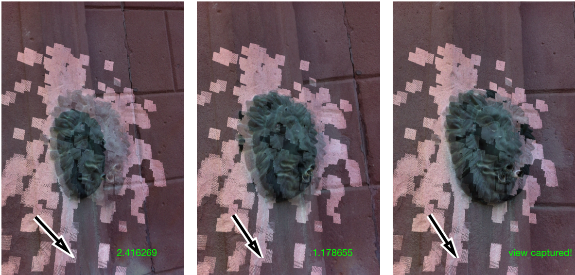
Figure 5: Capturing process for a specific view of the lion scene. The camera is moved according to the direction of the arrow, and finally aligns to the targeted position. The view is captured automatically.
