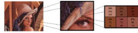
Figure 2: A digital image as a 2D discrete grid of pixels. In this case the cells contain 3 values of RGB color.
