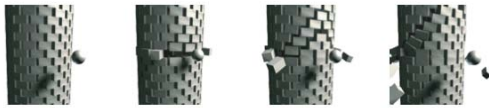
Figure 17: Test-cases that can reveal problems with freezing (sleeping policies). If too aggressive bricks will hang unnaturally in the air.
