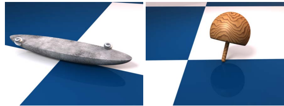
Figure 18: Rattleback (left) and tippe top (right) are good test cases for correct handling of gyroscopic forces.
