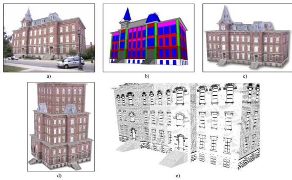
Figure 15: Example of inverse procedural modeling of a building from a photograph (top) and the application of the grammar to generate novel building variations (bottom). Figure or [ARB07], ©2007 IEEE.
