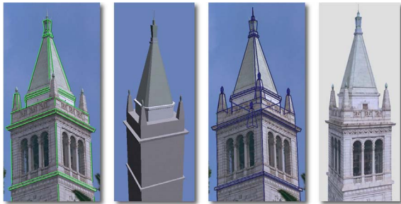
Figure 7: Interactive image-based modeling: (1) input image with user-drawn edges shown in green, (2) shaded 3D solid model, (3) geometric primitives overlaid onto the input image, (4) final view-dependent, texture-mapped 3D model. Figure courtesy of Paul Debevec [DTM96] ©1996 ACM.
