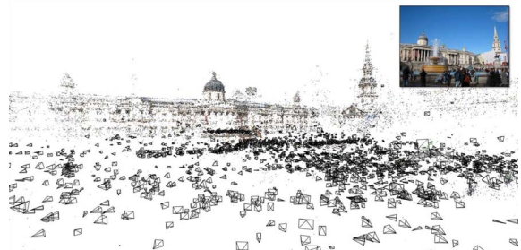
Figure 5: A sparse point cloud generated from several thousands of unordered photographs, and one photo taken from the nearly the same viewpoint. Figure courtesy of Noah Snavely [SSG*10], ©2010 IEEE.
