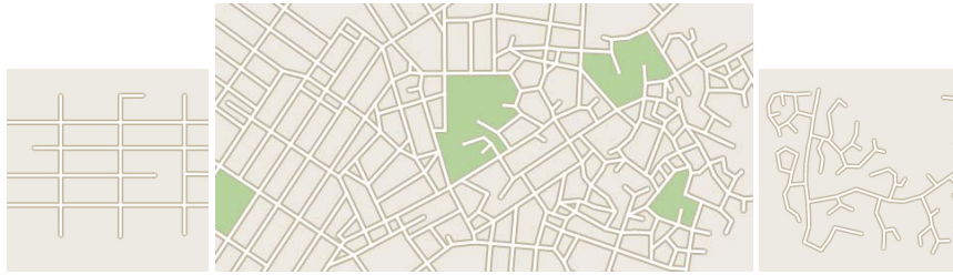
Figure 5: Given a grid example (left) and a curve example (right), our method synthesizes a new road network gradually varying from grid pattern to curve pattern from left to right (middle). Given a normalized x coordinates of a node being processed, we choose the grid example when f < x , and choose the the curve example when f > x , where f is a uniformly distributed random number between 0 and 1.
