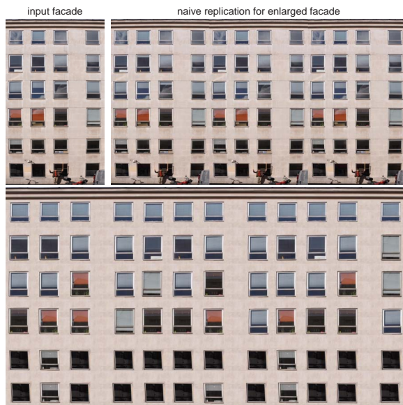
Figure 4: Starting from a single facade sample (top-left), we use our variation-factored representation to create procedural facade faces with variations (bottom-row).
