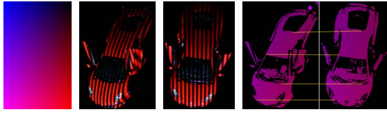
Figure 2: Left to right: The projected \Phi_x/\Phi_y (red/blue), fringe encoding, \phi_i/\phi_j with exemplary correspondences for two cameras C_i, C_j .
