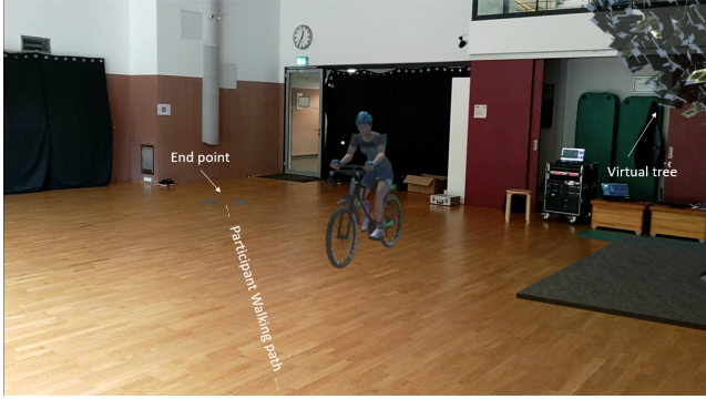
Figure 3: Mixed reality view of the crossing cyclist as seen from the HoloLens. The figure shows the walking path along with the virtual tree that was added to the scene.
