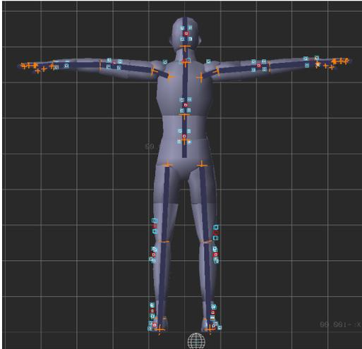
Markers are placed mostly on the back using a modular system featuring 3D printer cases.
