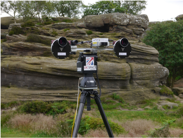
Figure 2: AUPE, the Aberystwyth University PanCam Emulator, during a field trial at Brimham Rocks, Yorkshire.
