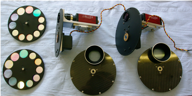
Figure 4: Partially-dismantled WACs, showing the filter wheels, front of the wheel housing with protective baffles, and rear of the housing fixed to the cameras.
