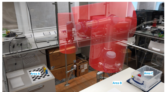
Figure 9: Sectional cylinder safety zone with hardware and network latency layer. The viewpoint is changed in this figure to show the position of the robot arm with respect to the table. Areas A, B and C are also labelled.
