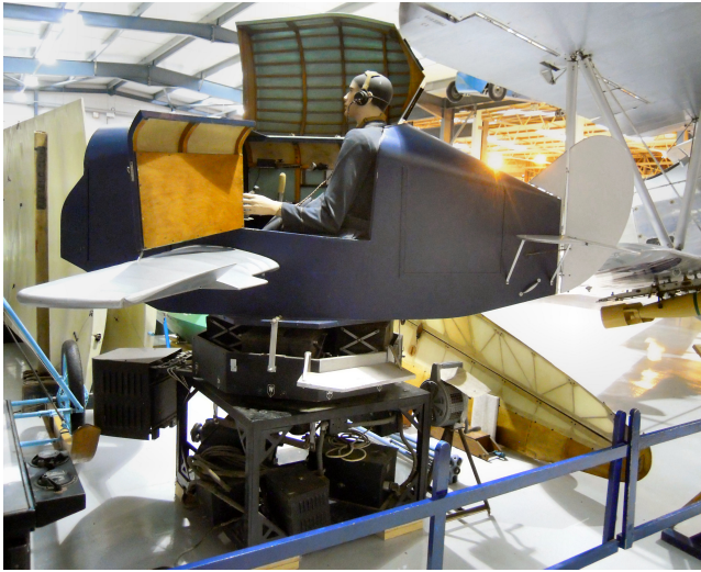
Figure 1: An example image of Link's trainer, one of the first moving-base flight simulators.
