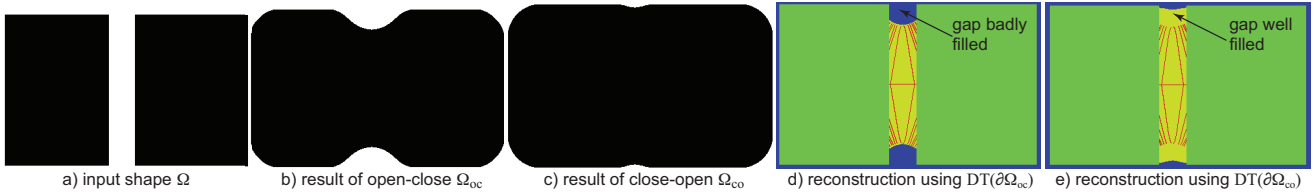
Figure 2: Effect of using distance transform of close-open shape \Omega_{co} vs distance transform of open-close shape \Omega_{oc} . See Sec. 3.3.
