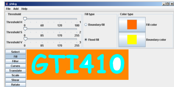
Figure 6: Results of a boundary fill from the contour of the image. The initial background is white.
