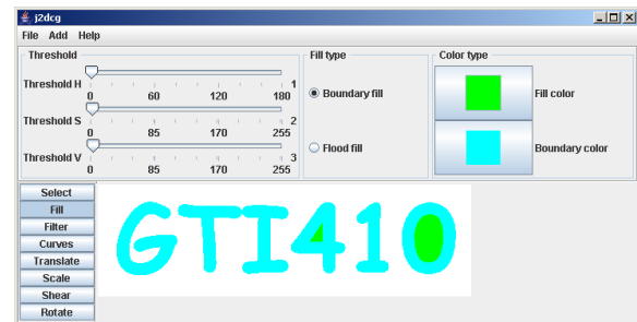
Figure 5: Results of a boundary fill inside the “4” and the “0”. The initial background is white.
