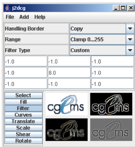
Figure 7: Different types of range mapping operations where values outside of 0..255 must be mapped back to 0..255 for display. Images left to right and top to bottom: original image, Laplacian filter with values clamped to 0 and 255, Laplacian filter with values transformed by computing their absolute value before mapping them to 0..255 (i.e. mapping the smallest value to 0 and the highest value to 255), Laplacian filter with values mapped to 0..255 (i.e. mapping the smallest value to 0 and the highest value to 255, without computing the absolute value).
