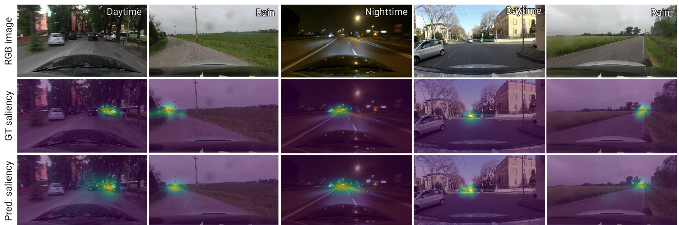
Figure 1: We present a convolutional recurrent encoder-decoder network for saliency prediction in driving scenes. Its convolutional structure allows for spatial reasoning, while its recurrent nature is well suited for learning the temporal dependencies of visual behavior in driving scenarios. It takes a sequence of RGB driving frames (first row) as input, and returns a sequence of predicted saliency maps (third row). We train different instances for varied weather and illumination conditions (namely daytime, nighttime, and rain), so that each of them is able to learn the particularities of the conditions. Our results are close to the ground truth (second row), and clearly outperform previous state-of-the-art approaches.
