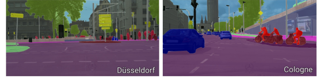
Figure 4: Visualization of semantic segmentation for two images corresponding to Düsseldorf (left) and Cologne (right) [COR*16]. Each color represents a different semantic category. Semantic urban scene understanding is critical when driving [COR*16], and we therefore provide our model with semantic information as part of the input.
