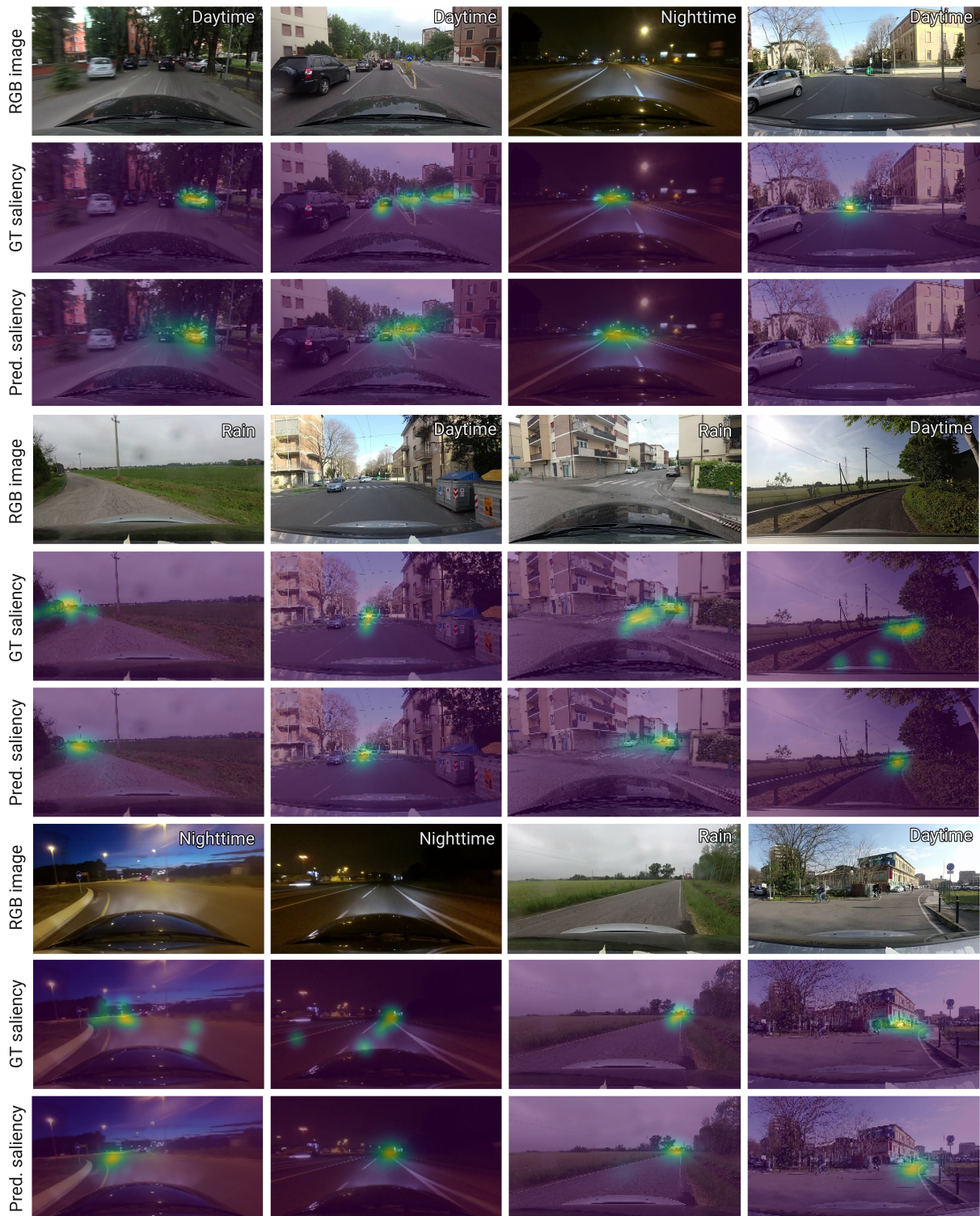
Figure 6: Qualitative results of our model. We show different saliency predictions in sets of three rows, where the first one depicts the original RGB frame, the second one corresponds to the ground truth (GT) saliency map, and the third one is the predicted (Pred.) saliency map. We include whether the image is from daytime, nighttime, or rain conditions (see Section 3.3) overlaid on the top-right of each RGB frame. Our predicted saliency maps closely resemble the ground truth ones, focusing on relevant parts, such as moving vehicles (first row, first column), or the streets the car is turning towards (third row, fourth column). Please refer to Table 2 for a quantitative evaluation.
