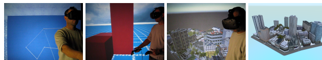
Figure 1: Our system allows inexperienced users to create complex cities in a few minutes. Users can design immersively both the street network and the overall shape and layout of buildings. Further detail is added through a procedural rule system.
