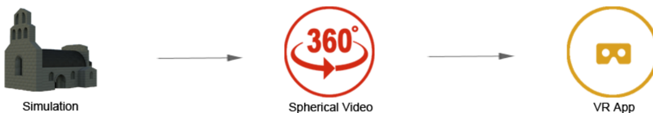
Figure 2: Our pipeline: A simulation is processed, and the resulting animation is rendered through a camera tailored for Virtual Reality. The 360° video obtained is exported to the Virtual Reality application that displays it on a headset.
