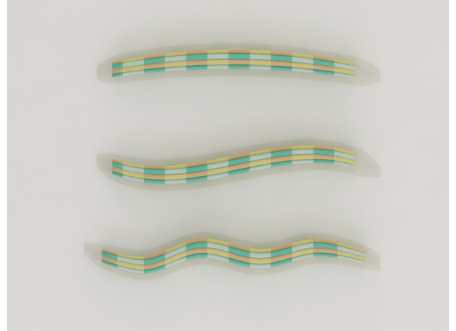
Figure 5: Several natural modes of our C. elegans model. From top to bottom: the 8 th , 10 th , and 16 th modes. We have selected the 10 th mode for our modal activation profile, as it produces one full undulation in the horizontal plane of the worm, and it resembles closely the undulation of C. elegans .
