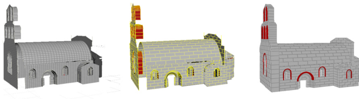
Figure 1: An input geometry of an ancient building like a church (left), is transformed by our interactive tool in a mesh of stone bricks (middle). Then, we added, through procedural modeling, the volume in the result geometry and the physical features for structural simulation (right). Colors on the final model were added for aesthetic purposes, following actual historic patterns.
