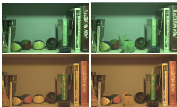
Figure 10: Spectrally-rendered Stanford bunny inserted in a scene illuminated with a green low-energy consumption light (top row) and a yellow incandescent (bottom row).
