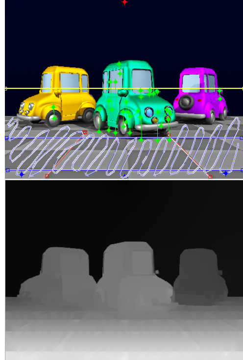
Figure 8: Equality constraints: depth map resulting from the addition of nineteen pairs of pixels (linked in green) with equal depth to the example in Figure 6.
