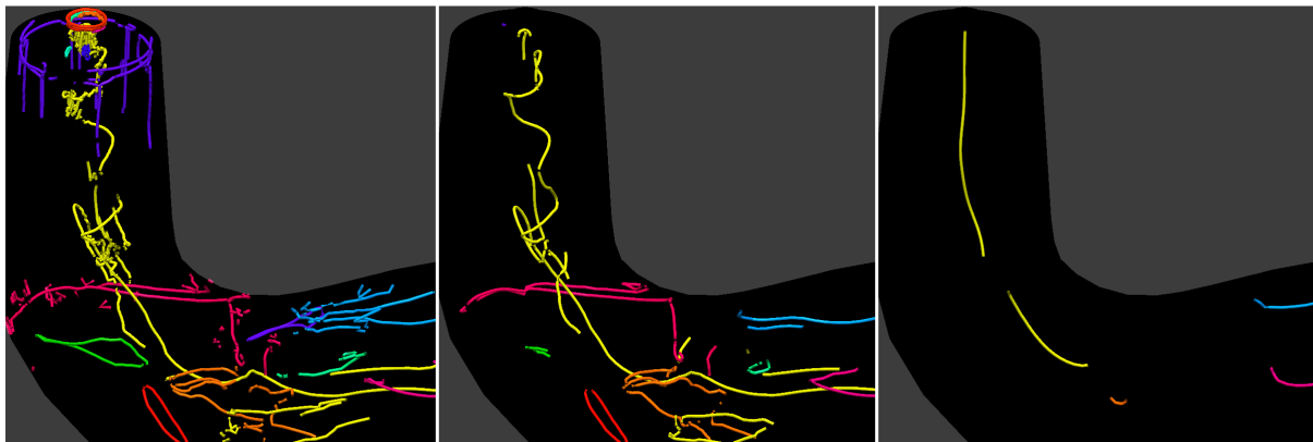
Figure 8: In the modernized draft tube, vortices are less articulate and harder to extract. Vortex core extraction based on normalized helicity has been applied to unsmoothed velocity field (left) and to Gaussian-smoothed data with \sigma=0.008 (middle) and \sigma=0.032 (right). Colors represent connected components of the surface swept by the core lines, see Fig. 9.
