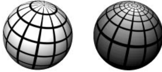
Fig. 1. Effect of the relativistic aberration of light on the texture mapped onto the unit sphere. The left sphere shows the mapping without distortion, the right sphere illustrates the distortion for 90 percent of the speed of light. The direction of motion shows towards the north pole of the sphere.
