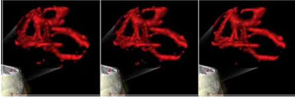
Figure 4: Different levels of smoothness at the super-resolution ROI. (Left) no subdivision, (middle) order 3 and (right) order 4 subdivisions.
