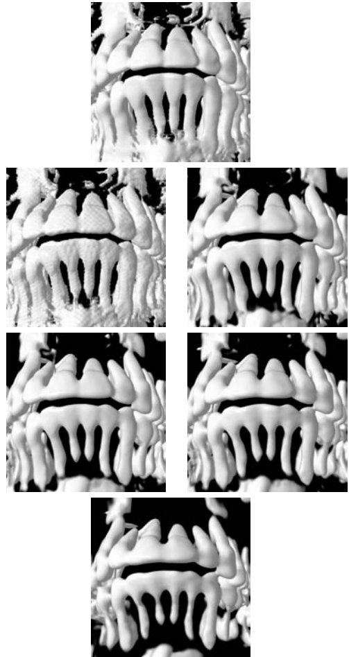
Figure 13: The skull data set at the original resolution of 128^3 at the top. First row, at half the resolution, left image on FCC, right on re-sampled Cartesian lattice. Second row at quarter resolution, left image on BCC and right image on re-sampled Cartesian. The bottom row, the dataset at one eighth resolution. These volumes are down-sampled using linear type filter and reconstructed using cubic type reconstructions.
