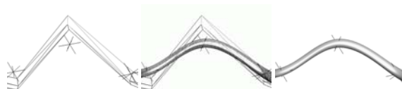
Figure 8: Computation of the base mesh. The stars show the positions of the C_\alpha atoms. While the generated base mesh does not need to include the C_\alpha positions, the spline curve that is generated at run time always does.
