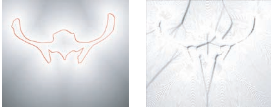
Figure 5: (left) Filtered Euclidean distance map that removes the medial-axis discontinuity. (right) A difference image calculated from Figure 4 (right) and Figure 5 (left) that highlights the pixels that have been modified by filtering.
