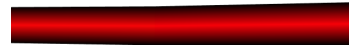
Figure 1: Tube-like rendering: result of view-vector oriented triangle strips with applied directional color coding for a single fiber.
